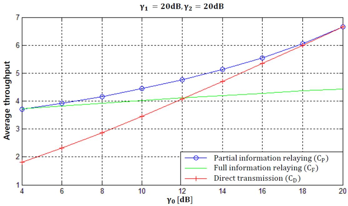
Figure 6. Achievable capacity of various relaying methods.
