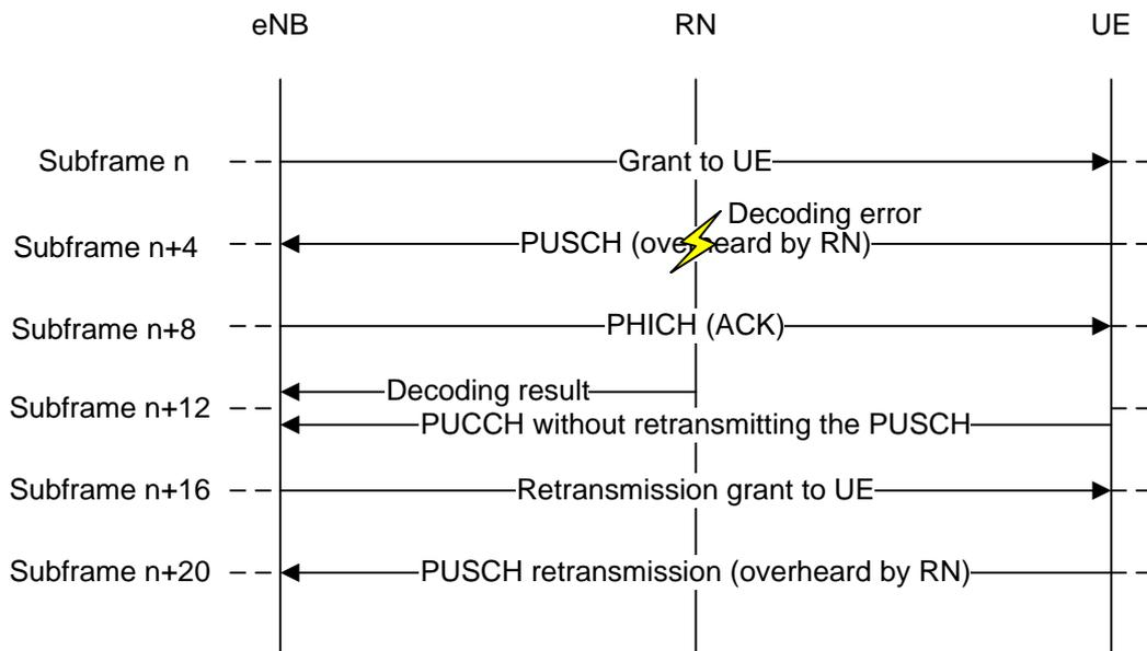
Figure 3. An example of RN's PUSCH decoding error recovery.
