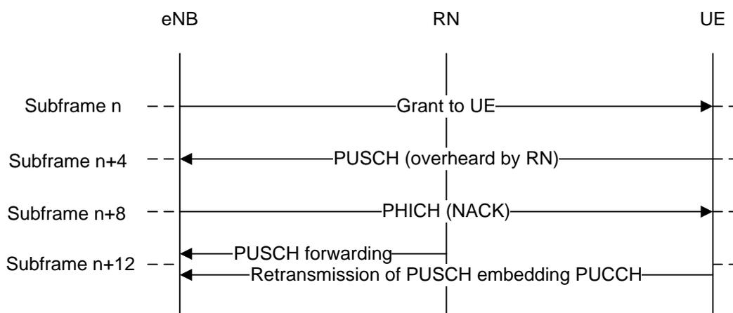
Figure 1. A problematic case in PUSCH forwarding in type II relay.
