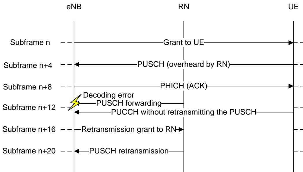
Figure 4. An example of eNB's PUSCH decoding error recovery.
