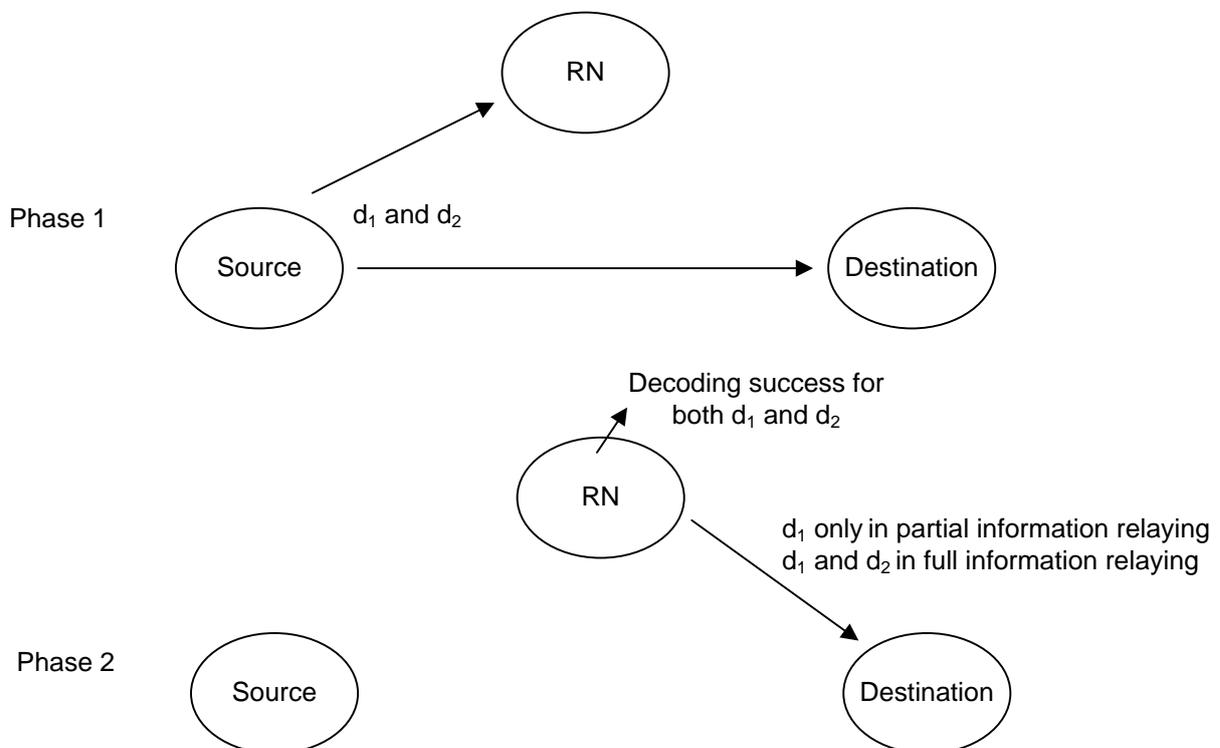
Figure 5. An example of partial information relaying for two data streams.
