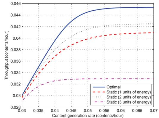
Fig. 3. Throughput under different content generation rate.
