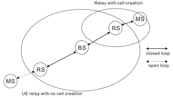
Fig. 1. The characteristics of UE relay
