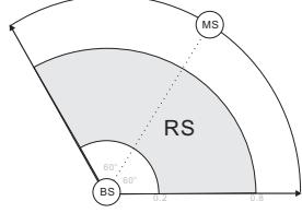
Fig. 6. Random MS placement: MS is randomly located in the shaded area
