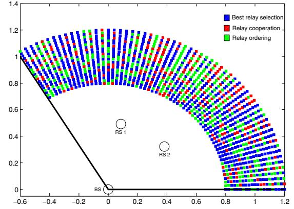
Fig. 11. The geometrical MS distribution associated with optimal relaying strategy when RSs are placed in the symmetric locations.
